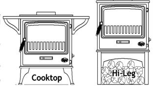
Attach to the underside of the stove using the bolts supplied before fully tightening. Note the 'Installation Clearances' on page 1. When used as a log store, logs must not be placed higher than the central 'bridging' member.
