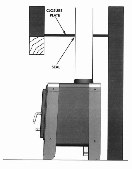
Typical Top Flue Installation using steel closure plate incorporating clean out door for chimney sweeping.
